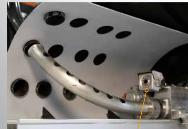
RUGGED CAMERA SYSTEM Facilitates quick indexing of boiler tubes
